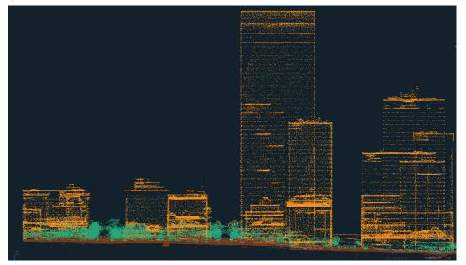
Use the Point Clouds feature to import and visualize large sets of point cloud data, such as 3D laser scanning/LiDAR data sets with millions of points.
