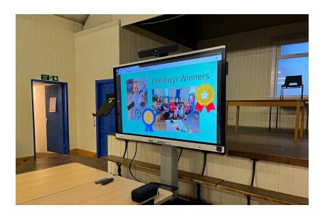
A SMART Board interactive whiteboard system, together with video conferencing camera/microphone/speaker system has been installed to provide a standalone touchscreen computing/hybrid meeting facility, with the option for users to connect their own devices to share and access content.
